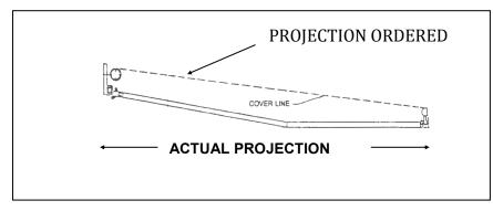
The SUNAIR® Lateral Arm Awning is designed for residential decks, patios and commercial storefronts. Smaller projections should be used for a storefront awning. The awnings are designed for sun protection; they are not designed to withstand wind or heavy rain and should not be sold for such purposes (see warranty).
