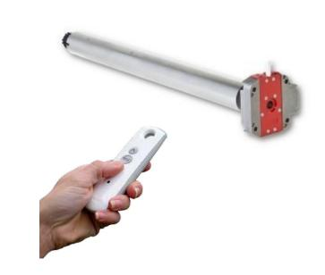
We offer a "Sunair" branded motor with our <u>Sunair® & Sunstar®</u> awning model awnings which is more economical. This motor is a 50 Nm radio RTS motor and is available on the above two models only. Maximum width using this motor is 28 ft. wide. This motor comes includes an 18' plug in cord and a one channel hand held remote. Somfy remotes and electronic controls are compatible and can be added.
