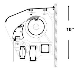
Sunair® offers an optional aluminum one piece hood, made from the highest quality aluminum. The hood protects the fabric when the awning is in retracted position. With the aluminum hood, your awning is always automatically covered when you retract it. If the awning is mounted under an overhang protruding at least 10", then the optional hood is not needed.
